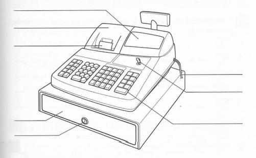
keyboard drawer lock mode switch power cord operator display printer cover receipt paper drawer
